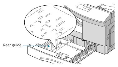
To remove and insert the rear guide, turn it slightly to your right side then lift it. While holding the rear guide at  $70^{\circ}$  angle, insert it into the corresponding position and push it to your left side until it stands up completely.
